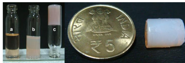
Figure 1. Photographs of gel formation (left) at (a) 1, (b) 3, and (c) 5 min and final monolith (right).
